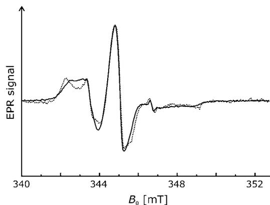
FIGURE 1 Comparison of normalized room temperature CW EPR spectra ( $T = 293$  K) of mutants H225R1 (solid line) and V254R1 (dotted line) recorded at pH 5.8. Differences in the signal/noise ratio are due to different concentrations of the samples.
