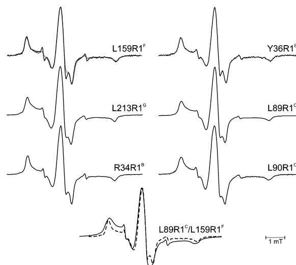
Figure 2. Room temperature first derivative cw electron paramagnetic resonance spectra of the MTS spin label attached to the indicated positions of the sensory rhodopsin NpSR II in complex with the transducer NpHtr II 157 reconstituted in purple membrane lipids (black lines). The spectra are scaled to equal positive amplitude of the central peak. The spectrum recorded for L159R1 F of NpSR II reconstituted in PML in the absence of NpHtr II (dotted line) is superimposed to the spectrum of L159R1 F in the 2:2 complex. At the bottom the dipolar broadened spectrum of the double mutant L89R1 C /L159R1 F (black line) is superimposed to the sum of the spectra of the corresponding singly labeled variants L89R1 C and L159R1 F (dashed line). Negligible amount of unbound spin label, which could not be eliminated by repetitive washing, is present in all spectra.
